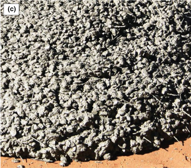
(100% recycled PP fibre dispersing in the fresh concrete
