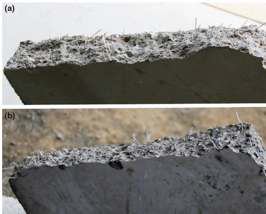
Fig. 5.9 Fracture faces of the PP fibres reinforced concrete round determinate panels: a line-indent PP fibre, and b diamond-indent PP fibre
