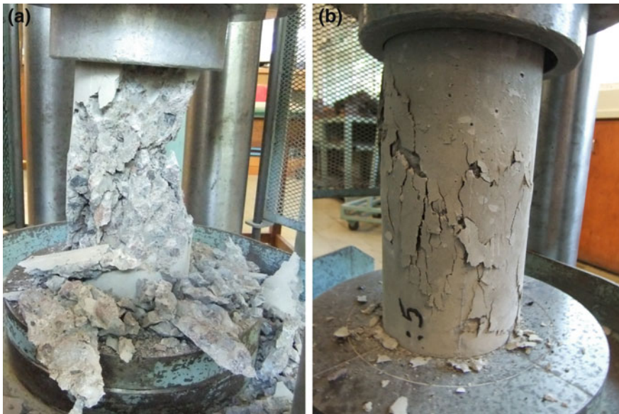
Fig. 4.10 Failure behaviour of a plain concrete and b fibre reinforced concrete in the compression test
